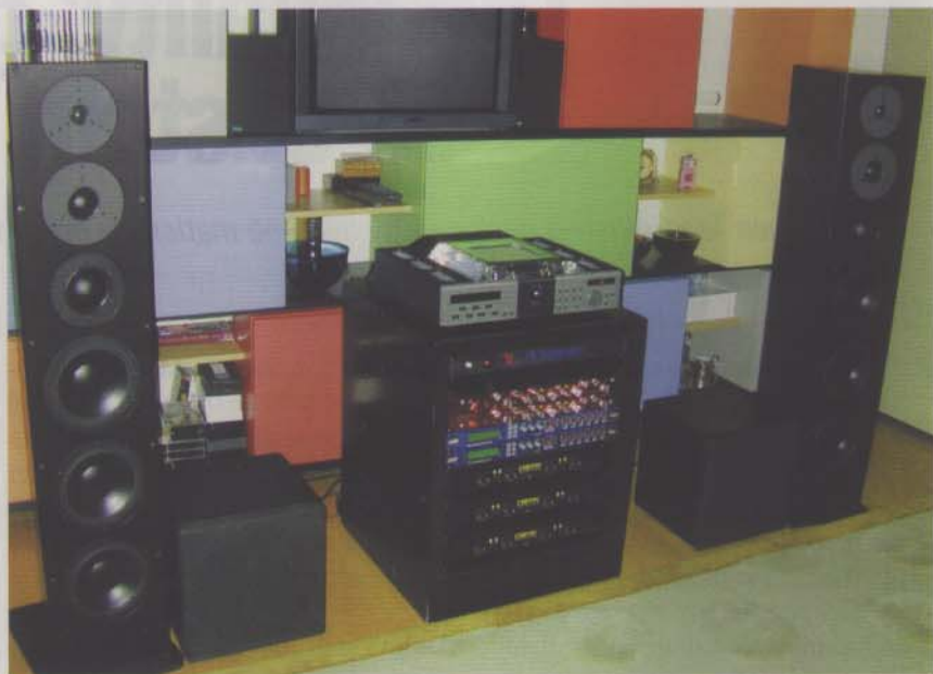
An early-stage consumer installation featuring a pair of Rothstein originals: custom-made floorstanding loudspeakers with anodized aircraft-grade aluminum front panels and wood cabinets. Special, laser-cut gaskets were designed to Rothstein's specifications to join the front panel to the speaker chassis for optimal sound reproduction. The TV was later replaced with a 50" plasma display
